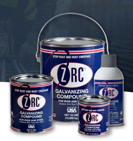
ZRC Cold Galvanizing Compound is an organic, single component zinc-rich coating which has 95% pure zinc metal in the dried film and is recognized by Underwriters' Laboratories, Inc. to be equivalent in corrosion protection to hot-dip galvanizing.
